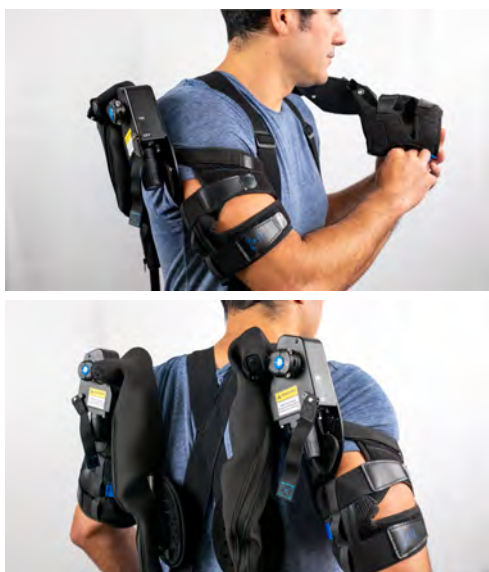
Figure 14: Installing Ekso EVO Suspenders
