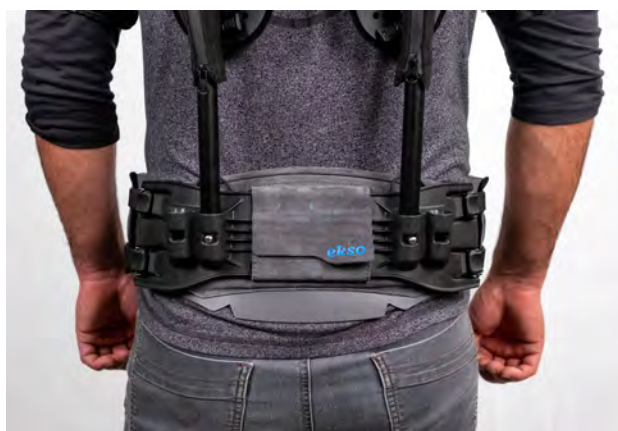
Figure 11: Ekso EVO in narrow position
