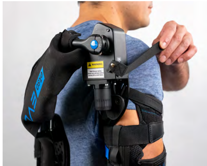
Figure 17: Turning Ekso EVO On
