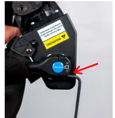
Figure 20: Loosening End Link Screw
