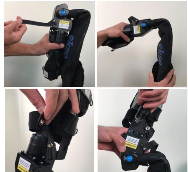
Figure 9: Installing Actuator Springs
