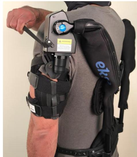
Figure 8: Turning EVO On
