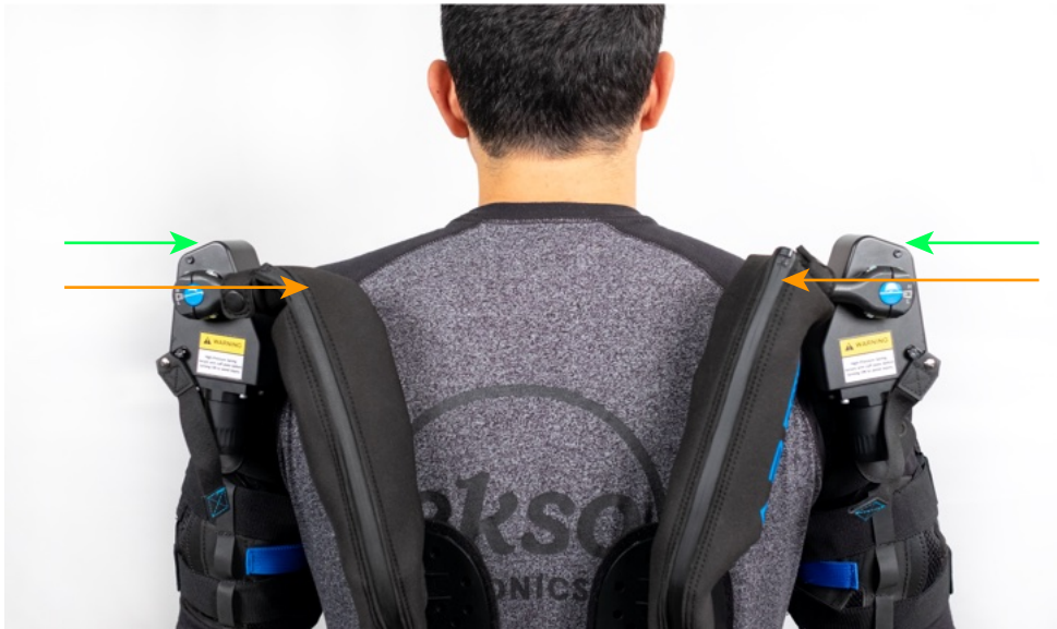
Figure 10: Proper Ekso EVO Actuator Height Alignment
